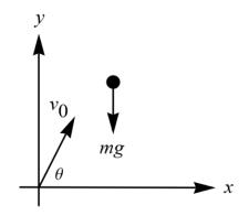
Newton's second law states that the sum of the forces on the ball is equal to its mass times acceleration.
